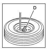
14. Tilt the retainer (D) at the end of the cable and pull it through the wheel opening. Pull the tire out from under the vehicle.
